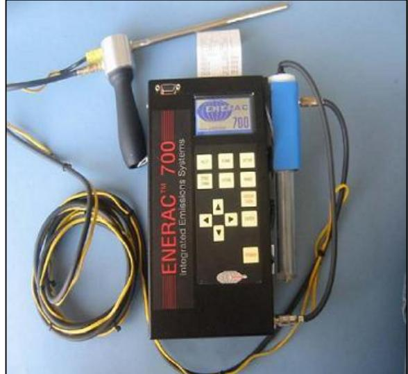
The image shows the ENERAC 700 Integrated Emissions System. It is a black handheld unit with a digital display showing '700' and a keypad with yellow buttons. Two yellow flexible hoses are connected to the front, leading to a probe assembly. The probe assembly includes a blue cylindrical component and a metal probe tip. The entire setup is resting on a light blue surface. |
