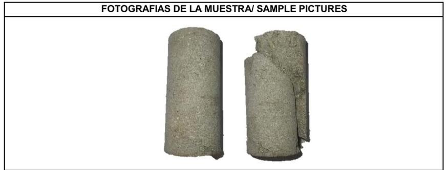
ESFUERZO MAXIMO/MAXIMUM STRESS 106.09 kg/cm<sup>2</sup> 10.40 MPa TIPO DE FALLA/FRACTURE TYPE: 2
