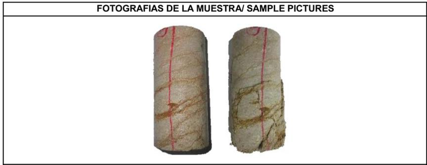
ESFUERZO MAXIMO/MAXIMUM STRESS 84.02 kg/cm<sup>2</sup> 8.24 MPa TIPO DE FALLA/FRACTURE TYPE: 3
