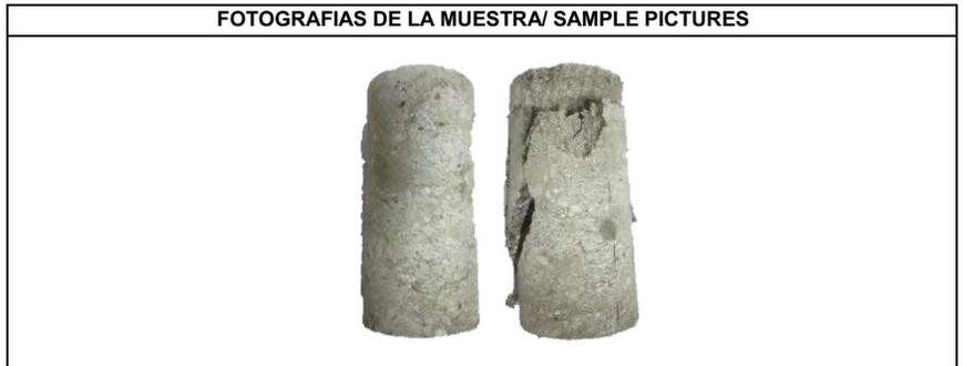
ESFUERZO MAXIMO/MAXIMUM STRESS 150.20 kg/cm<sup>2</sup> 14.73 MPa TIPO DE FALLA/FRACTURE TYPE: 2
