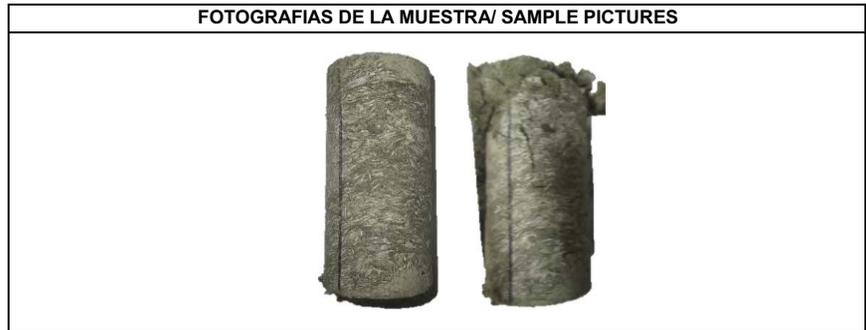
ESFUERZO MAXIMO/MAXIMUM STRESS 48.18 kg/cm<sup>2</sup> 4.73 MPa TIPO DE FALLA/FRACTURE TYPE: 3
