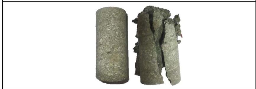
ESFUERZO MAXIMO/MAXIMUM STRESS: 112.09 kg/cm<sup>2</sup> 10.99 MPa TIPO DE FALLA/FRACTURE TYPE: 2
