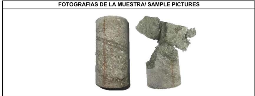
ESFUERZO MAXIMO/MAXIMUM STRESS 62.59 kg/cm<sup>2</sup> 6.14 MPa TIPO DE FALLA/FRACTURE TYPE: 3
