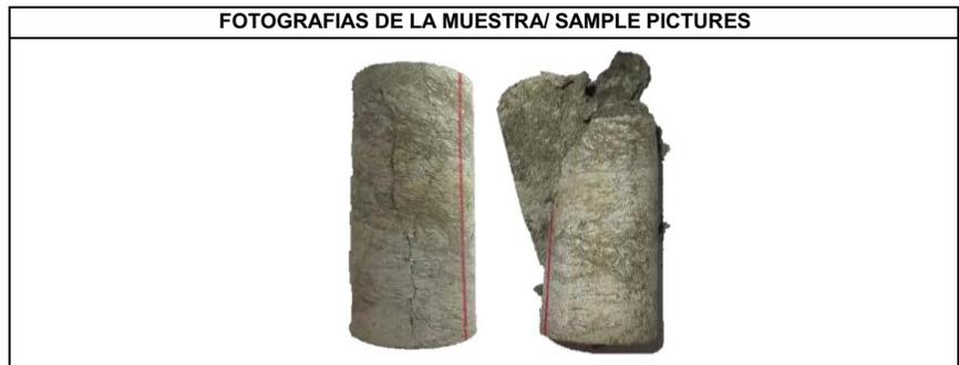
ESFUERZO MAXIMO/MAXIMUM STRESS 91.59 kg/cm<sup>2</sup> 8.98 MPa TIPO DE FALLA/FRACTURE TYPE: 2
