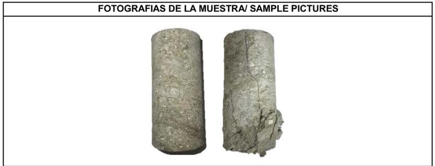
ESFUERZO MAXIMO/MAXIMUM STRESS: 104.74 kg/cm<sup>2</sup>      10.27 MPa
