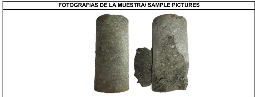
ESFUERZO MAXIMO/MAXIMUM STRESS 115.45 kg/cm<sup>2</sup> 11.32 MPa TIPO DE FALLA/FRACTURE TYPE: 2
