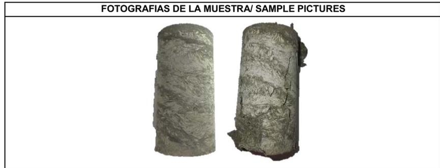
ESFUERZO MAXIMO/MAXIMUM STRESS 71.83 kg/cm<sup>2</sup> 7.04 MPa TIPO DE FALLA/FRACTURE TYPE: 2
