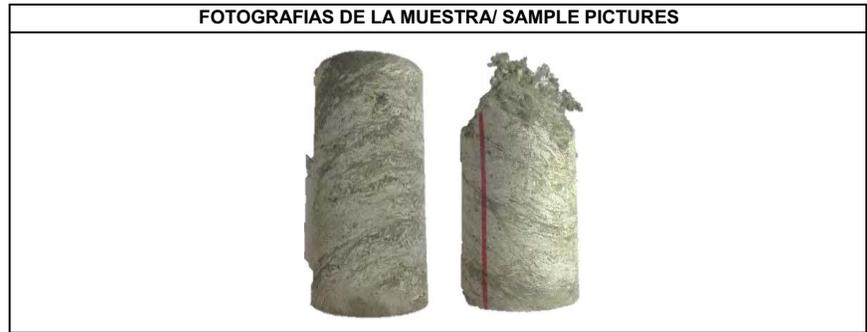
ESFUERZO MAXIMO/MAXIMUM STRESS: 48.31 kg/cm<sup>2</sup>      4.74 MPa      TIPO DE FALLA/FRACTURE TYPE: 4
