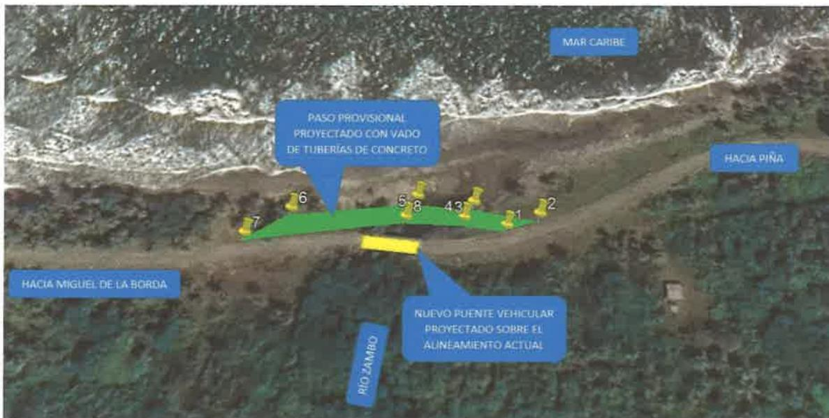
**Figura N°6 Paso Provisional Río Zambo**
