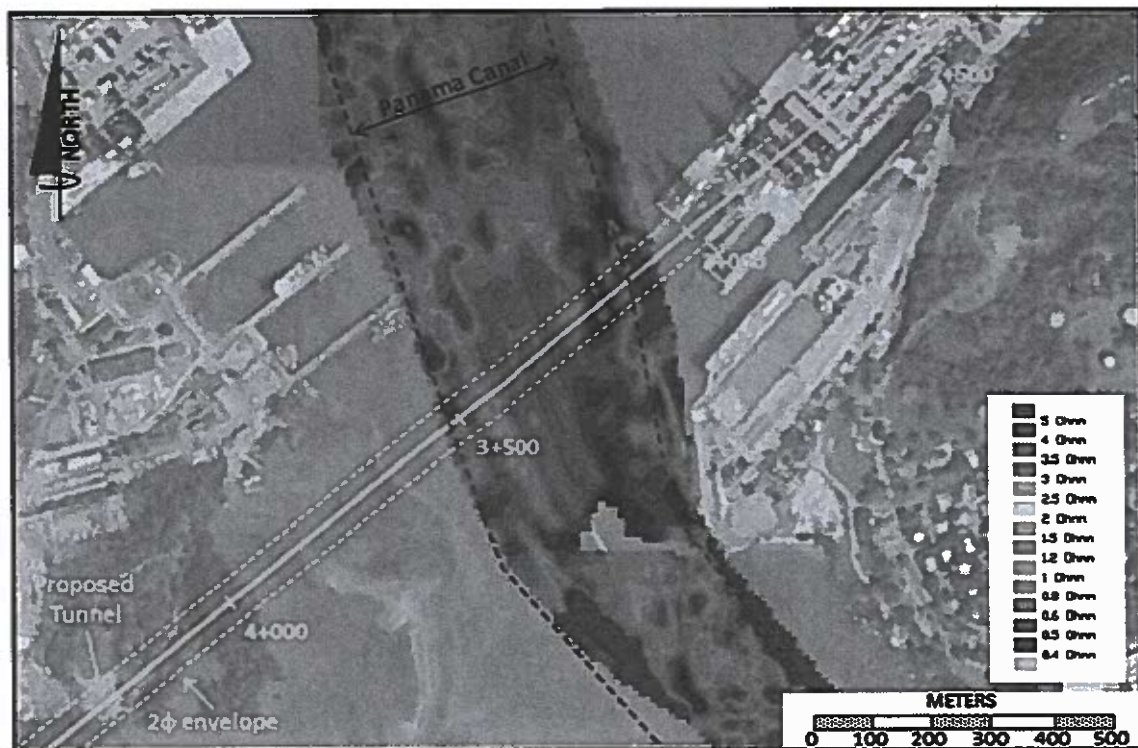
Figure 6: Resistivity Survey Along the Canal
