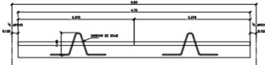
ELEVACION LATERAL DE VIGA LOSA AASHTO 2.00mX0.25m
