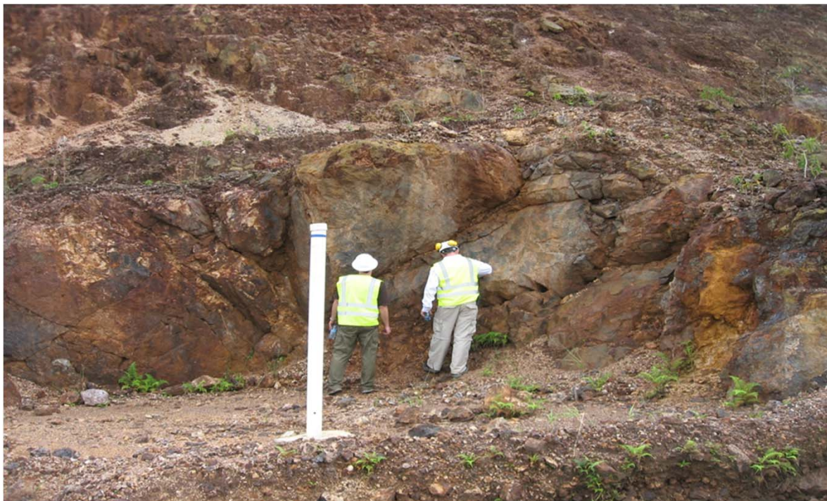
PHOTOGRAPH 20 MODERATE STRENGTH, BLOCKY ROCK IN LA PAVA AREA
