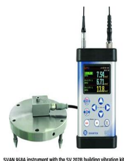
SVAN 958A instrument with the SV 2078 building vibration kit
