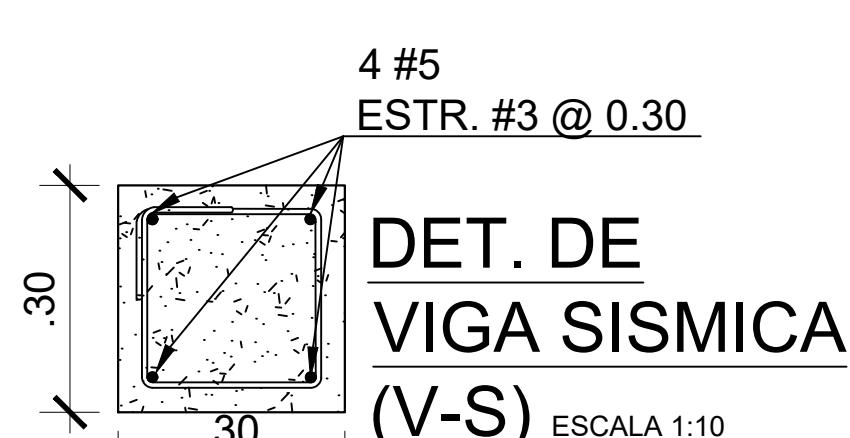
**DET. DE VIGA SISMICA (V-S)** ESCALA 1:10
