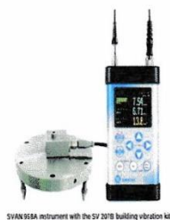
SVAN 958A instrument with the SV 2018 building vibration kit
