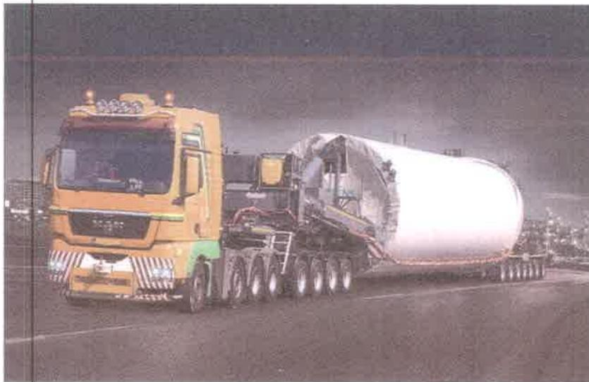
FIGURA 22. EJEMPLO DE VEHÍCULOS PORTA TUBOS (TORRES) TIPO MEGA WINDMILL TRANSPORTER.
