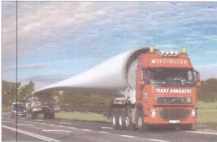
FIGURA 21. SEMIRREMOLQUE TIPO SUPER WING CARRIER.
