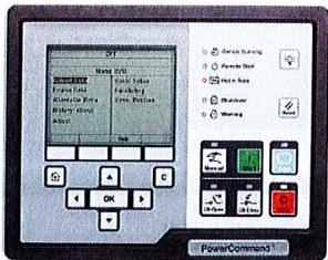
The PowerCommand control system is an integrated microprocessor based generator set control system providing voltage regulation, engine protection, alternator protection, operator interface and isochronous governing. Refer to document S-1567 and S-1570 for more detailed information on the control
