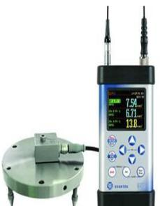
SVAN 958A instrument with the SV 207B building vibration kit
