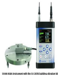
SVAN 80A instrument with the SV 2070 building vibration kit
