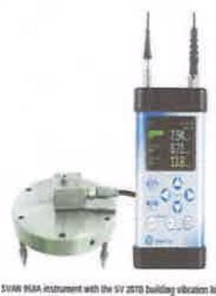
SV 8400 LMA instrument with the SV 2070 building vibration kit
