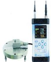
The image shows the SVAN 858A instrument, which is a handheld device with a color screen and various buttons, connected to a circular vibration probe. Below the instrument is its carrying case, labeled 'SV 2018 building vibration kit'.
